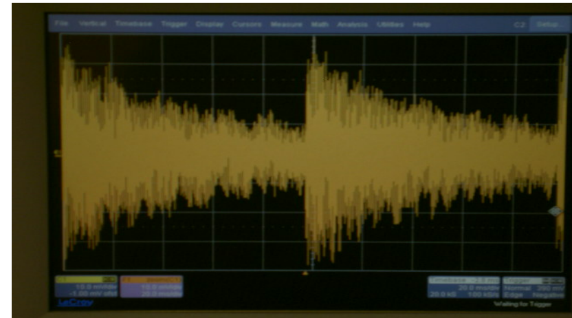
synchrotron light from a bending magnet in MAX I (20 ms/division)
